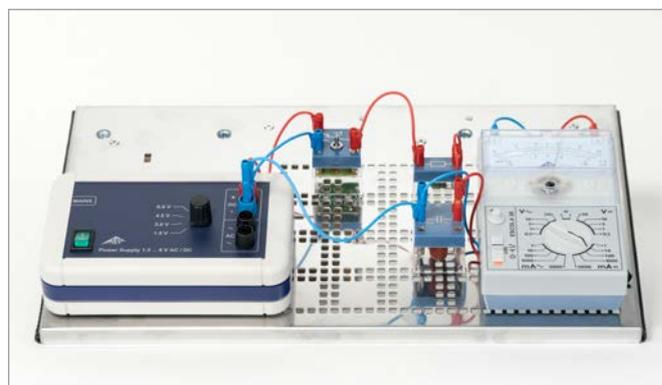
Charging and discharging of a capacitor (voltage)
