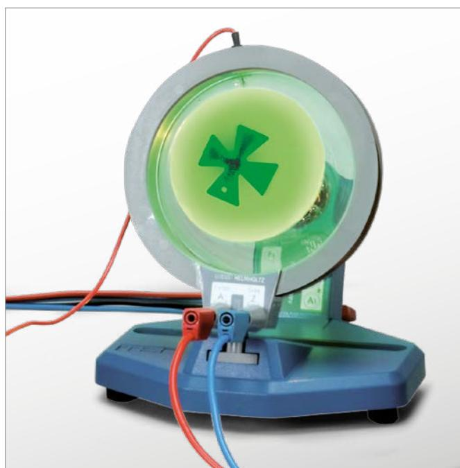
Fig. 2: Rotation of the electron shadow through deflection of electrons in the axially aligned magnetic field
