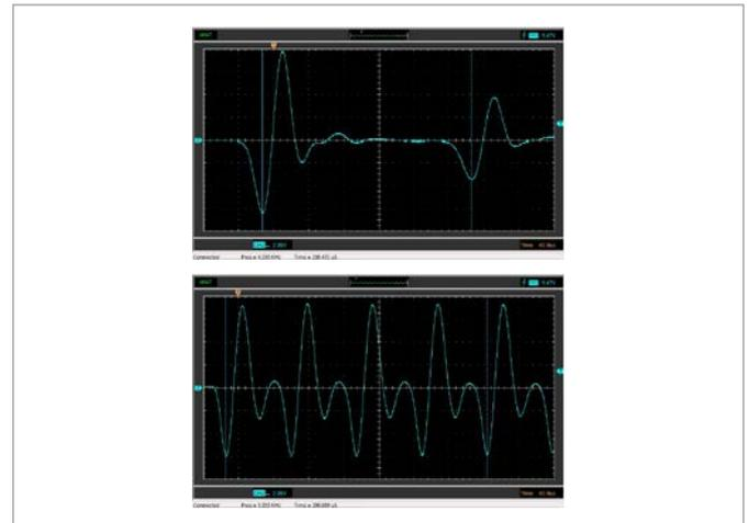
Fig. 3: Propagation of a sound pulse (top: PVC rod, 200 mm, bottom: glass rod, 200 mm), signal at the opposite end of the rod from the excitation (cyan)
