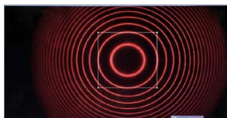
Fig. 2: No external magnetic field: Observation of the interference rings of the red cadmium line created by the Fabry-Pérot etalon. As an orientation aid, the second interference ring from the centre is indicated with a frame.
