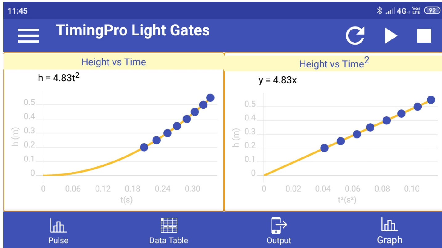
Timing-Pro Light Gates app : Plot of h \sim t and h \sim t^2 can be obtained in an android or iOS smartphone when a single light gate is used at various positions
